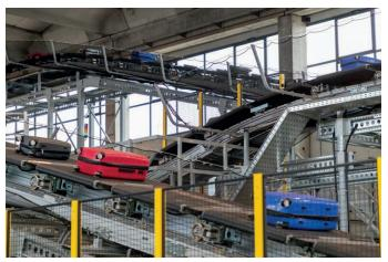
> The aluminum rails are coated with stainless steel in order to minimize the friction with the rolling wheels.
